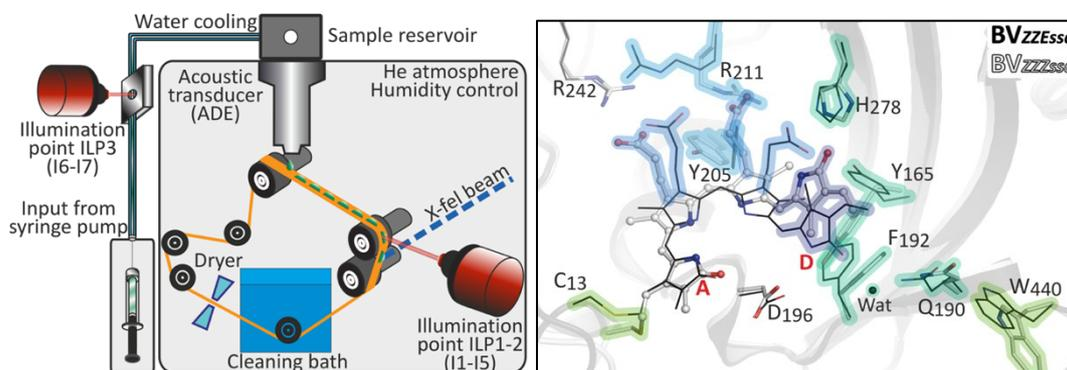
**Figure 1:** Sample delivery system specific for XFEL measurements (**left**) and close-up view on the chromophore binding pocket to illustrate of time-resolved structural changes (**right**).
